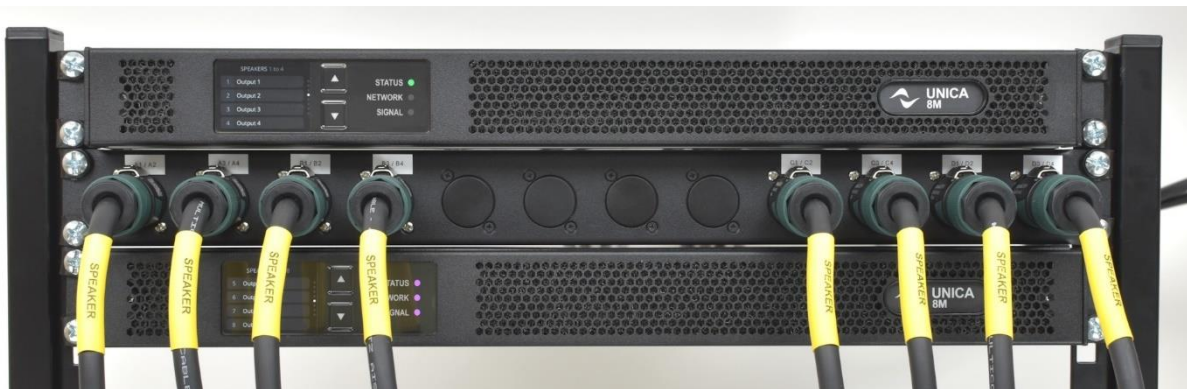
Figure 4.6 - KET setup with 16 channels / 2 Unica with KET Unica Patch-Bay – front side
