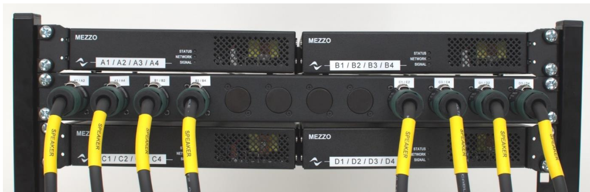
Figure 4.4 - KET setup with 16 channels / 4 Mezzi with KET Mezzo Patch-Bay – front side
